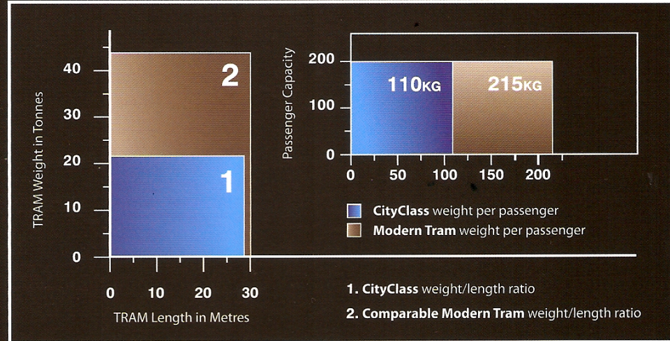
THE COMPARISON GRAPH SHOWS CITYCLASS WEIGHING 50% LESS THAN A SIMILAR SIZED MODERN TRAM
