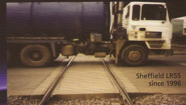
Deflection under 25 tonne axle load
